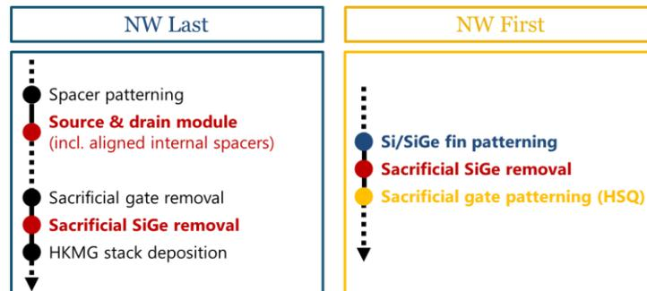
Figure 3.23 – Steps involving SiGe selective removal in NW first and in NW last approaches (red color).
