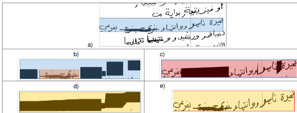
FIGURE 4.9: MADDCAT line delimiter ground truth e) derived from word delimiters ground truth b) c)
