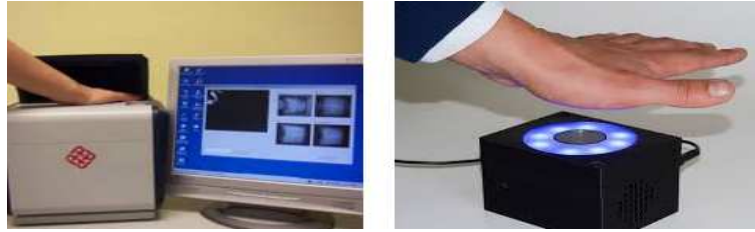
FIGURE 3.5: Examples of palmprint acquisition devices [Zhang 2010].
