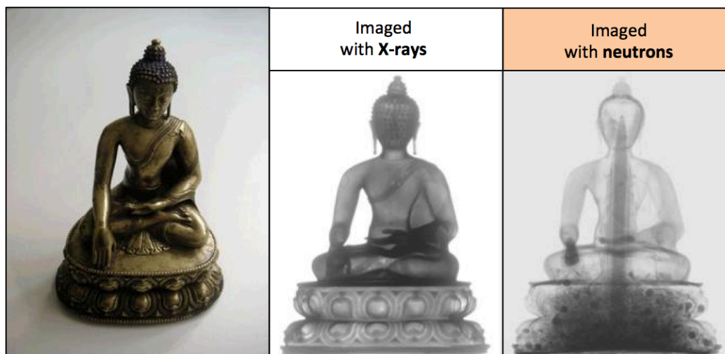
Figure 1.5 Study of the inner content of Buddha sculptures. Photo: example of Sakyamuni, Bhumisparśa Mudra, West Tibet, 14 th –15 th century. The left X-ray radiography doesn't show content while the right neutron radiography provide information about the embedded organic material. Taken from [Lehmann 2010].
