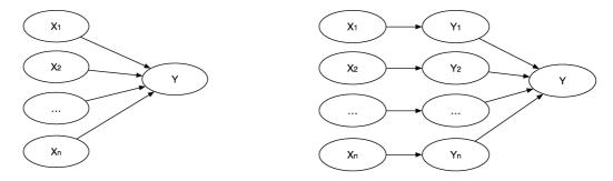
Figure 3-4: Convergent connexion of node
