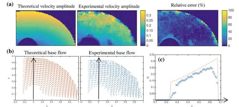
**Figure 4.** Comparison between the theoretical base flow in (8) and (9) and the PIV measurements. (a) Velocity amplitude. (b) Velocity field. (c) Velocity amplitude as a function of the  $y$  position for  $x=0$ . The dashed orange line represents the theoretical velocity amplitude, and the blue circles represent the experimentally measured velocity.
