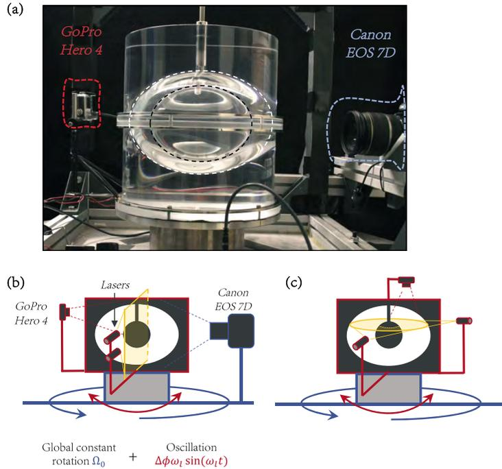
**Figure 2.** (a) Side view image and (b, c) schematic representations of the laboratory experiment used to perform visualizations on vertical and horizontal planes. The inner core is spherical, even if it appears ellipsoidal in Figure 2a due to optical distortions.
