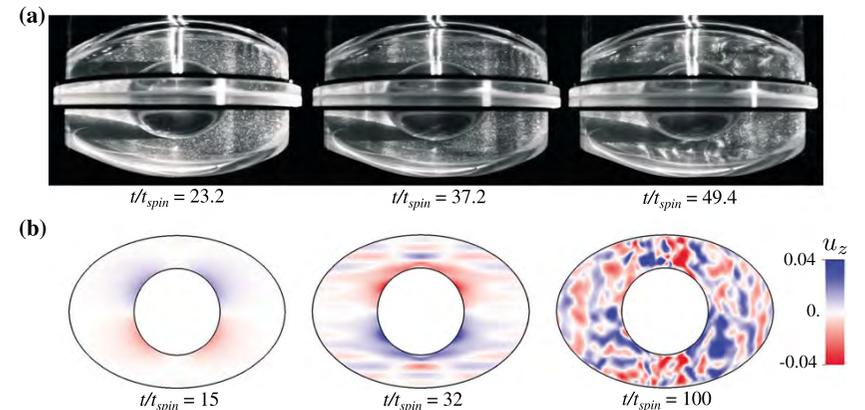
**Figure 7.** Comparison of the onset of LDEI for laboratory experimental and numerical simulations through meridional side view visualizations at  $E_\chi = 10^{-4}$ ,  $f = 4$ ,  $\epsilon = 0.35$ , and  $\chi = 0.49$ . (a) Experiments: Kalliroscope visualizations made in the rotating frame. (b) Numerical simulations: the vertical velocity is shown through snapshots made in the librating frame.
