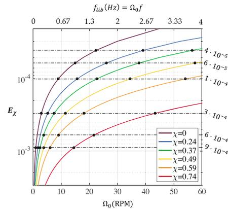
**Figure 3.** Evolution of the Ekman number with the rotation rate of the turntable for various shell ratios. The black dots represent the cases realized for a dimensionless libration frequency  $f = 4$ .
