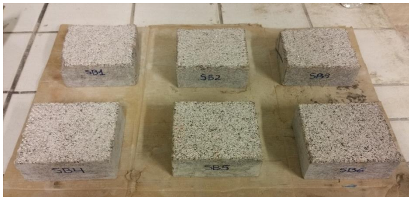
Figure 3.27: Surface texture of bush-hammered samples ready for shear testing
