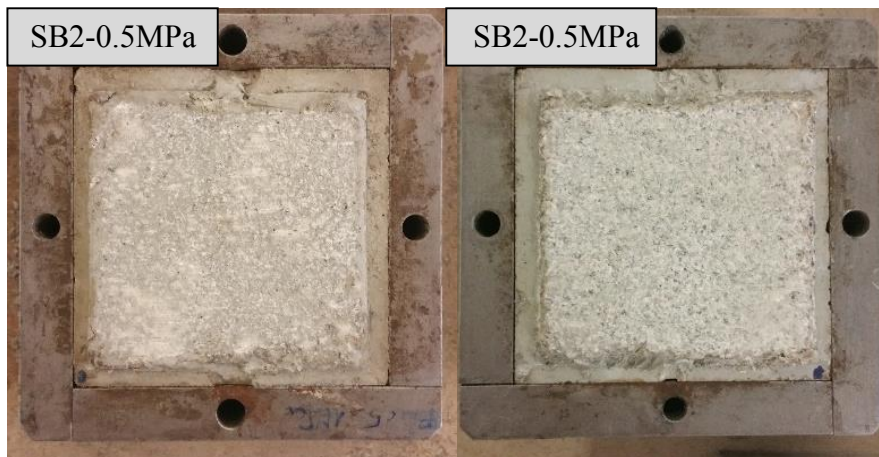
Figure A.11: Photos of the bush-hammered sample SB2 after the shear test conducted at 0.5MPa of normal stress (left: concrete, right: granite)
