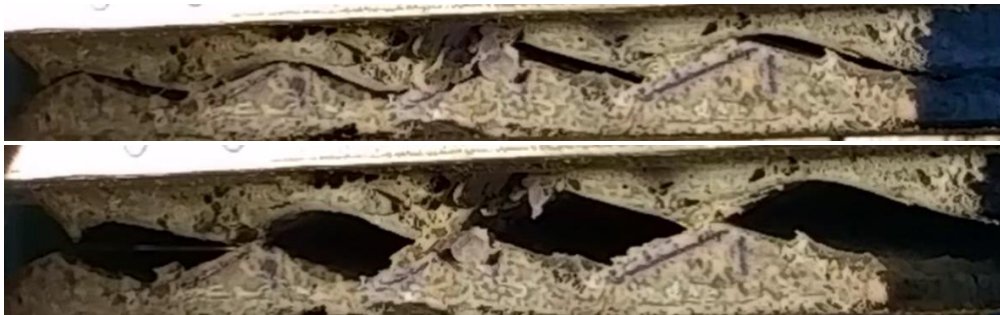
Figure 4.4: Photos of the tooth-shaped asperities for the test 2 conducted under \sigma_n=1\text{MPa} during the ascending phase. Sliding is the governing shearing mechanism: no damage of the concrete asperities can be observed
