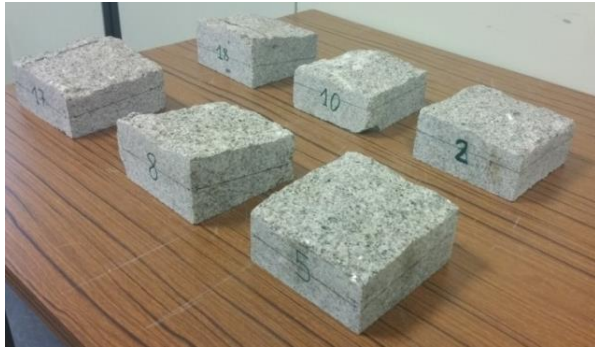
Figure 3.12: Planes parallel to the discontinuities mean plane are drawn on the specimens
