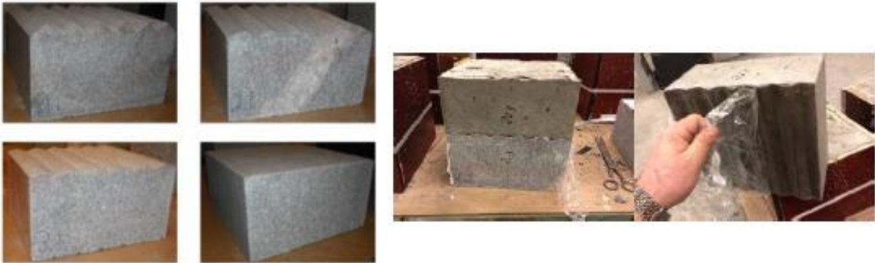
Figure 2.21: Surface profiles tested and plastic film removal before shear tests
