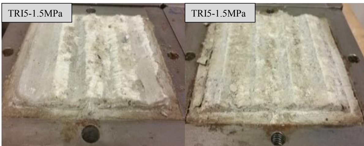
Figure B.7: Photos of the sample 5 with tooth-shaped asperities after the shear test conducted at 1.5MPa of normal stress (left: concrete, right: granite)
