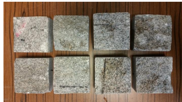
Figure 4.10: Natural granite samples before (a) and after (b) cleaning with water
