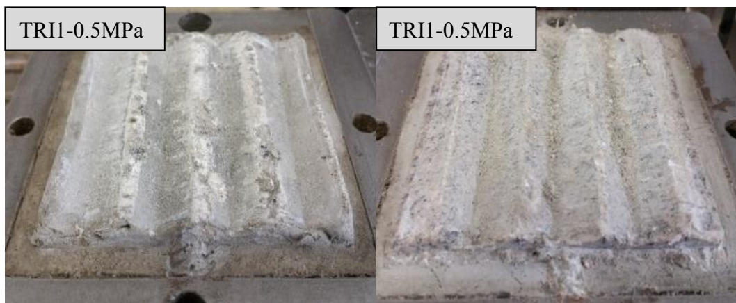
Figure B.4: Photos of the sample 1 with tooth-shaped asperities after the shear test conducted at 0.5 MPa of normal stress (left: concrete, right: granite)
