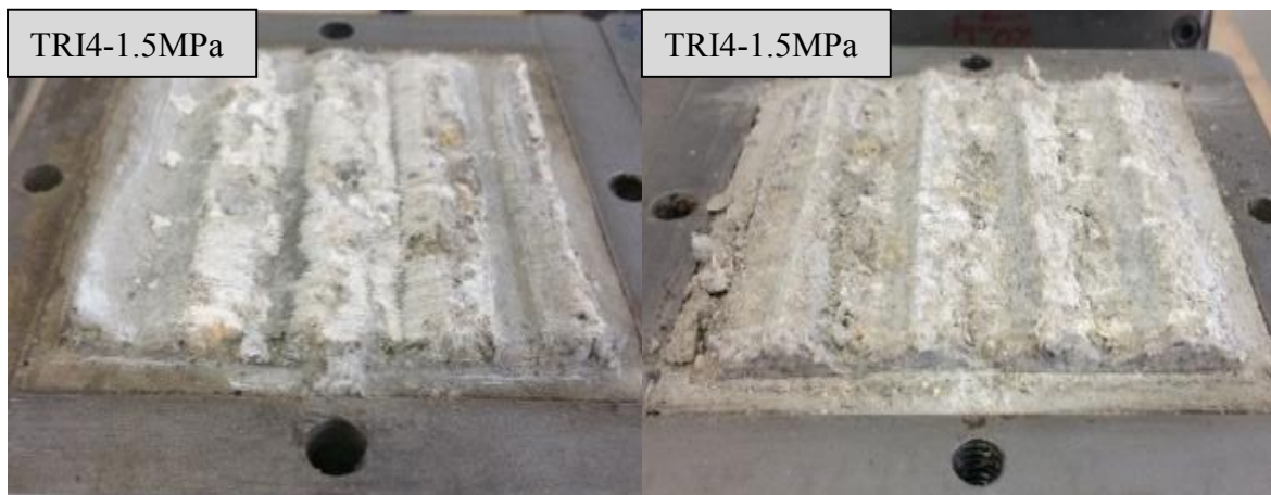
Figure B.6: Photos of the sample 4 with tooth-shaped asperities after the shear test conducted at 1.5MPa of normal stress (left: concrete, right: granite)
