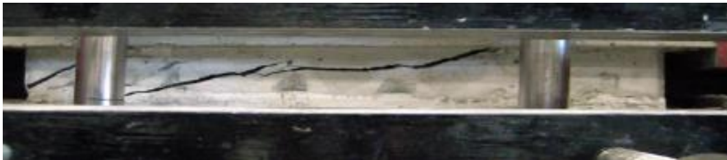
Figure 2.23: Failure of a bonded specimen with i=40^\circ and \sigma_n=1.2 MPa.
