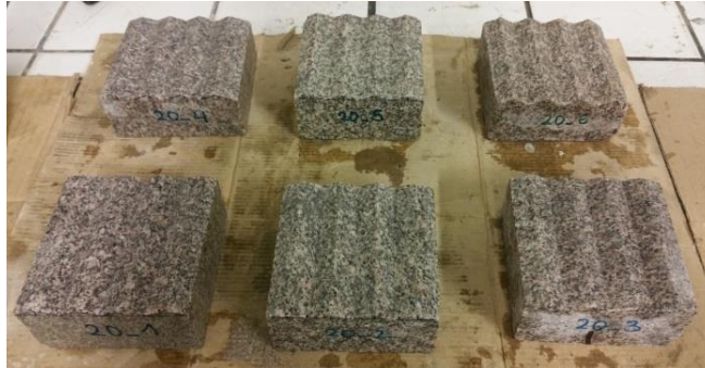
Figure 4.2: Granite samples cleaned with water before the preparation of the shear boxes
