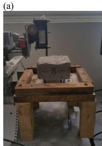
Figure 3.14: (a) Adjustment of the position of the specimen so that the mean plane is horizontal, (b) Scan after the procedure was put into place
