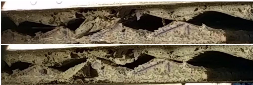
Figure 4.5: Photos of the asperities for the test 2 conducted under \sigma_n=1\text{MPa} during the descending phase: slight damage and shearing of the tip of the concrete asperities can be observed while the granite surface remains intact
