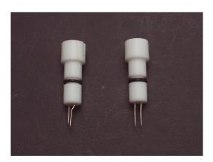
**Figure 3.3:** Picture of two home-made PTFE electroformation caps with different gaps between the platinum electrodes, (left) 1 mm and (right) 2.5 mm.
