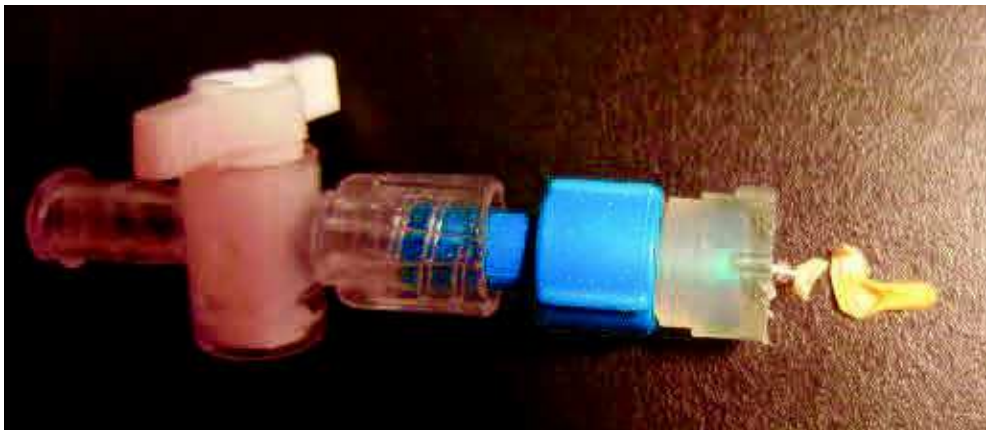
Figure 15: Polyisoprene balloon 4 weeks after inflation with saline
