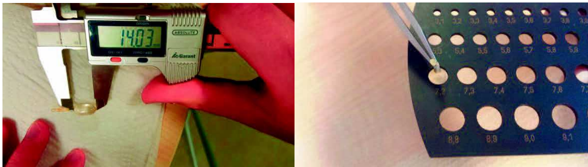
Figure 36: Methods for measurements of length and diameter of the balloon
