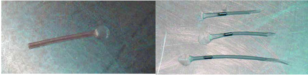
Figure 16: Distal end forming of latex free balloons by tube welding
