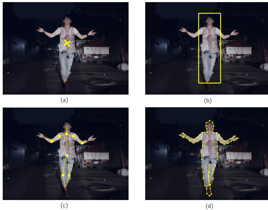
FIGURE 1.1: Common object representations: (a) Centroid, (b) Bounding Box, (c) Skeleton and (d) Object Contour.
