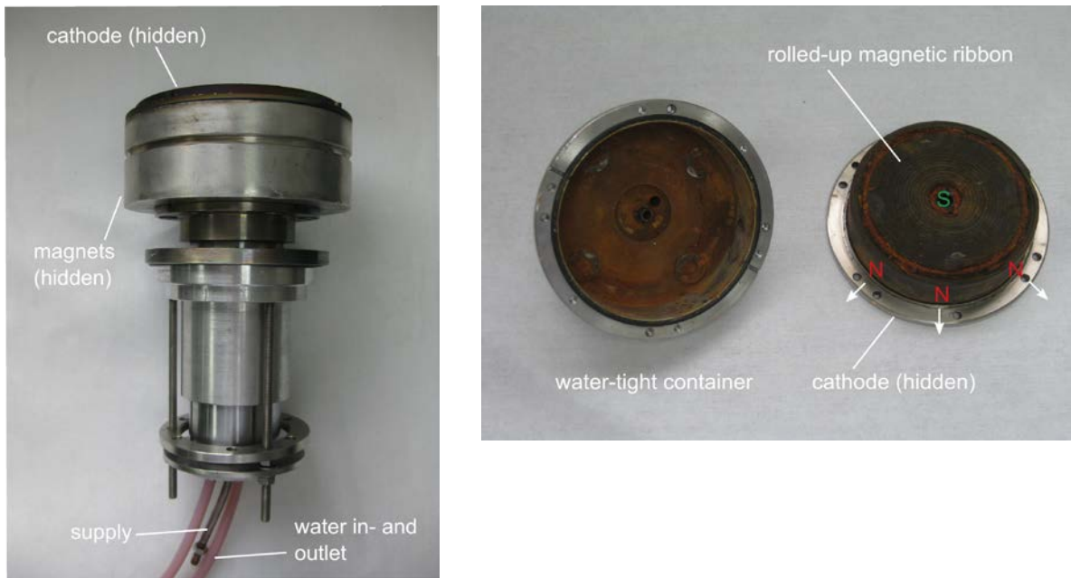
Fig. 41: Left: Assembled magnetron. Right: Opened-up magnetron showing the rolled-up magnetic ribbon.
