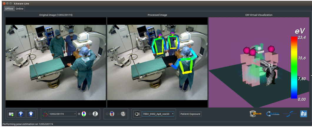
Figure 7.2: Clinician tracking in XAware-Live : the 2D body-joints' positions are overlaid over the color image (left) and the persons' 3D positions are shown in a virtual environment (right).
