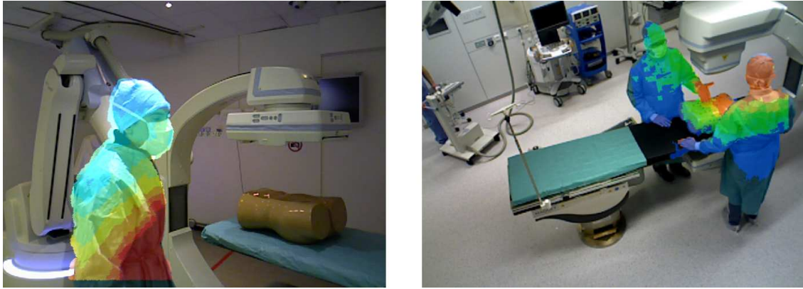
Figure 5.6: (Left) Mobile AR visualization of a clinician’s exposure during a PA projection. (Right) Ceiling-view AR visualization of the exposure of two clinicians for an AP projection.
