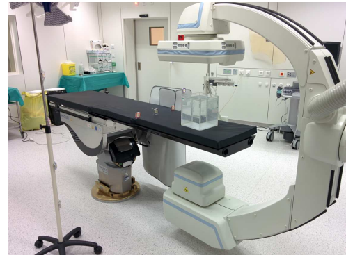
(b) Setup for experimental validation performed at IHU Strasbourg: PA imaging projection, water-filled slab phantom and wireless dosimeters.
