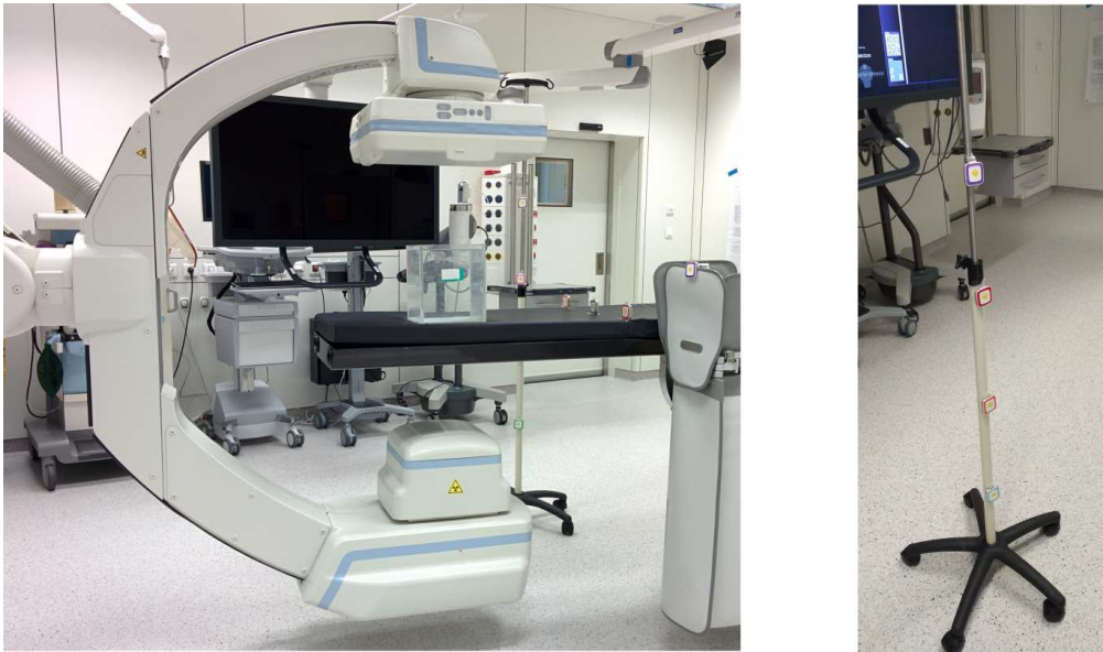
Figure 6.7: (Left) Setup for the dose measurements performed in a hybrid OR at IHU Strasbourg using a Siemens’ Artis Zeego X-ray imaging device and RaySafe dosimeters. (Right) Four dosimeters taped to a drip rod used to obtain dose measurements over a “dummy” clinician’s body.
