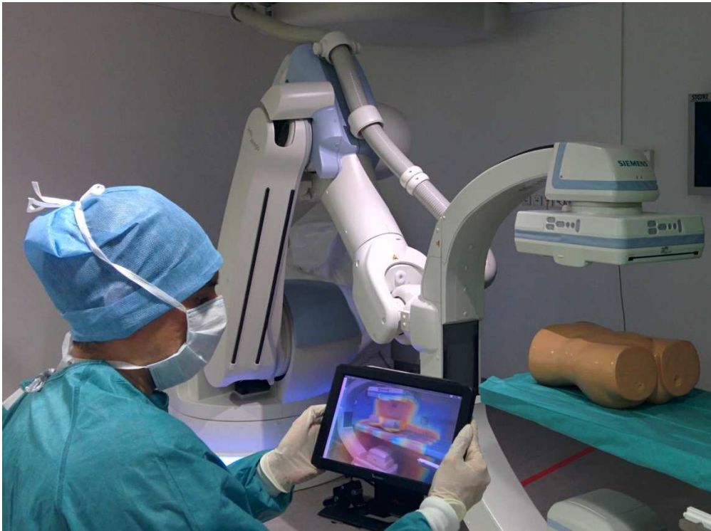
Figure 5.7: Mobile AR visualization for radiation awareness using a hand-held screen. The user visualizes the propagation of scattered radiation for the current device configuration directly in his own view.
