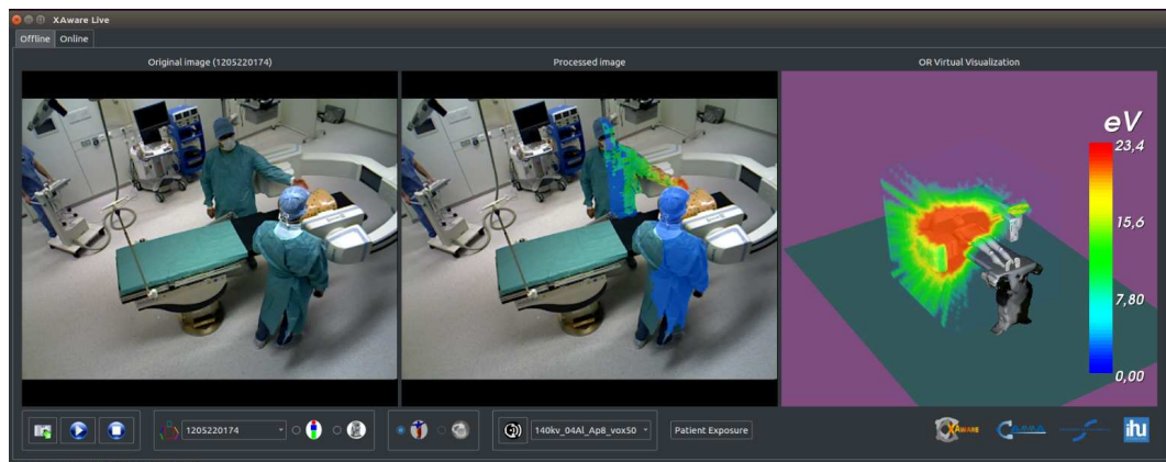
Figure 7.5: AR visualization of the current personnel’s body radiation exposure with XAware-Live .
