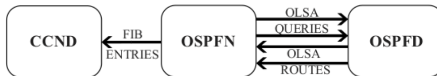
Figure 3.1: Relationship between CCND, OSPFN and OSPFD, from [35].
