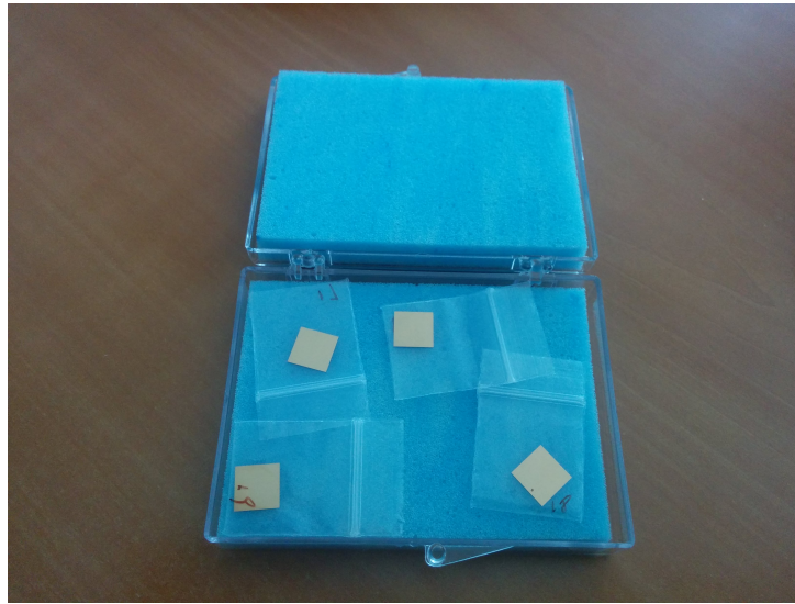
Figure 4.5 – Individual PMN-PT substrates obtained from CTG Advanced materials, delivered with Au/Cr electrodes.
