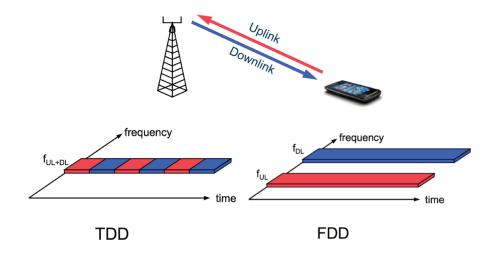
Fig. 2.7 Frequency- and time-division duplex. Source: [3]
