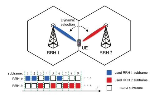
Fig. 2.16 A simple example of dynamic point selection with two cooperative RRHs.
