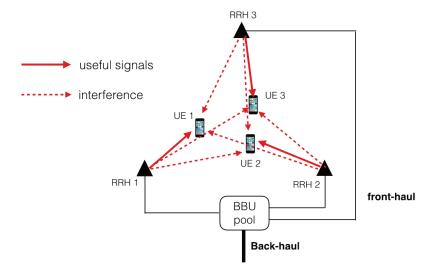
Fig. 5.1 Downlink transmission scheme of single RRH mode.
