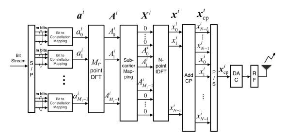
Fig. 3.1 Localized DFTS-OFDM transmitter.
