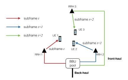
Fig. 5.5 Downlink transmission scheme of round robin selection.
