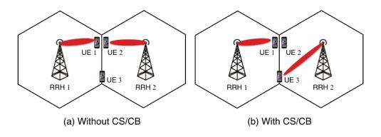
Fig. 2.17 A simple example of cooperative scheduling/cooperative beamforming with two cooperative RRHs.
