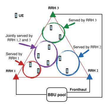
Fig. 7.1 An example of hybrid transmission.
