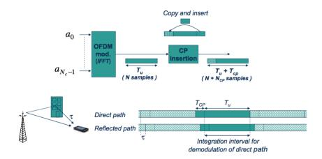
Fig. 2.3 Cyclic-prefix insertion. Source: [3]
