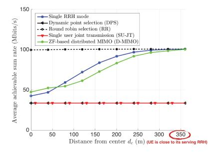
Fig. 5.16 Average achievable sum rate vs. UE distance from the center of RRH 1, 2 and 3  $d_c$  with small fronthaul capacity ( $P_{\rm dBm}=41.4~{\rm dBm}, \overline{C}=33.6~{\rm Mbits/s}$ ).
