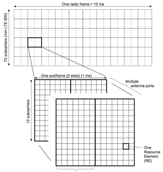
One Physical Resource Block (PRB) with  $N_{\text{symbol}}$  OFDMA/DFTS-OFDM symbols ( $N_{\text{symbol}} = 7$  if normal CP is applied,  $N_{\text{symbol}} = 6$  if extended CP is applied)
