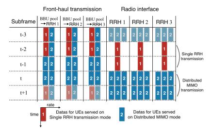
Fig. 7.6 Fronthaul transmission with previous data transmission for the UEs served in distributed MIMO mode.
