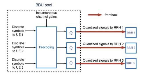
Fig. 2.20 Downlink compression after precoding (CAP) transmission scheme ("Q" represents compression).
