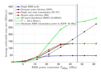
Fig. 5.13 Average achievable sum rate vs. RRH power constraint  $P_{\rm dBm}$  ( $\overline{C}=134.4$  Mbits/s,  $d_{\rm c}=0$  m).
