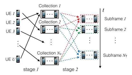
Fig. 6.2 Process of allocating UEs to be served in different subframes with UDA.
