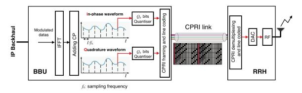
Fig. 2.12 The CPRI interface protocol for *IQ* data transmission from BBU to RRH in LTE downlink.
