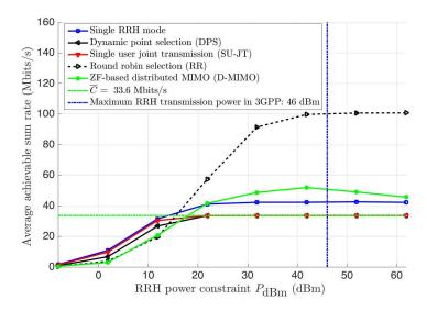
Fig. 5.14 Average achievable sum rate vs. RRH power constraint  $P_{\rm dBm}$  with small fronthaul capacity ( $\overline{C} = 33.6$  Mbits/s,  $d_{\rm c} = 0$  m).
