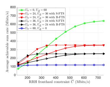
Fig. 7.10 Comparison of average achievable sum rate vs. fronthaul capacity constraint  $\overline{C}$  for different transmission strategies (no zoom).
