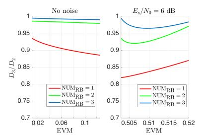
Fig. 3.10 The relative transmission data rate between method 2 and 3 with respect to the same value of EVM.
