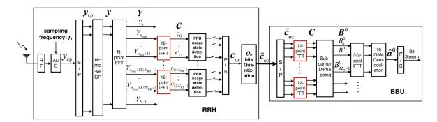
Fig. 3.6 Method 3 of functional split between RRHs and BBUs.
