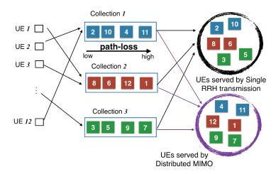
Fig. 7.3 Process of separating UEs to twos parts, some served in single RRH mode and the others in distributed MIMO mode.
