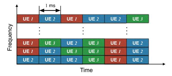
Fig. 2.4 Example of resource allocation in LTE.
