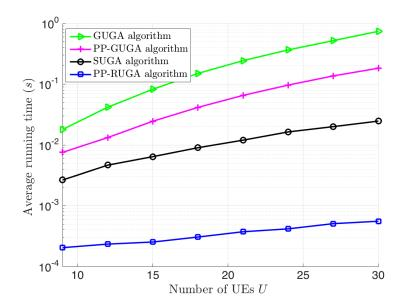
Fig. 6.8 Running time vs. number of UEs U ( $P_{\rm dBm} = 46$  dBm,  $Q_{\rm q} = 4$ ).
