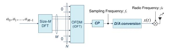
Fig. 2.5 DFTS-OFDM signal generation. Source: [3]
