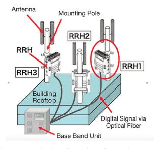
Fig. 2.10 Typical configuration of eNB. Source: [4]
