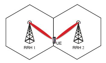
Fig. 2.18 A simple example of Joint Transmission with two cooperative RRHs.
