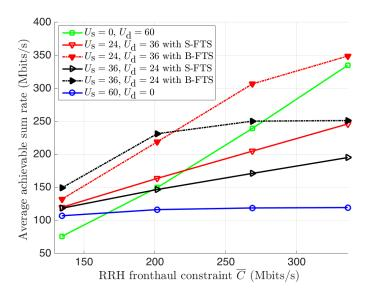
Fig. 7.11 Comparison of average achievable sum rate vs. fronthaul capacity constraint  $\overline{C}$  for different transmission strategies (zoom).
