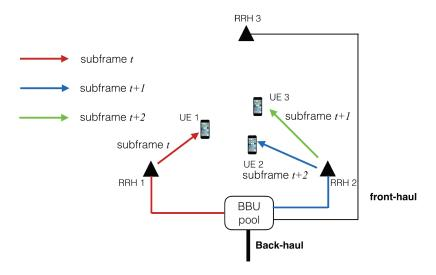
Fig. 5.3 Downlink transmission scheme of dynamic point selection.
