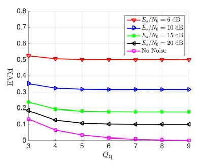
Fig. 3.8 EVMs for applying method 1 of receiver with different  $(\frac{E_s}{N_0})_{\rm dB}$  and quantization resolution  $Q_{\rm q}$ .
