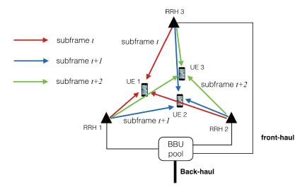
Fig. 5.7 Downlink transmission scheme of single user joint transmission.
