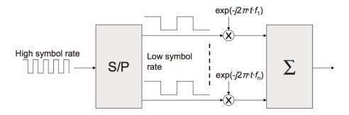
Fig. 2.1 Principle of transmission in OFDM. Source: [2]
