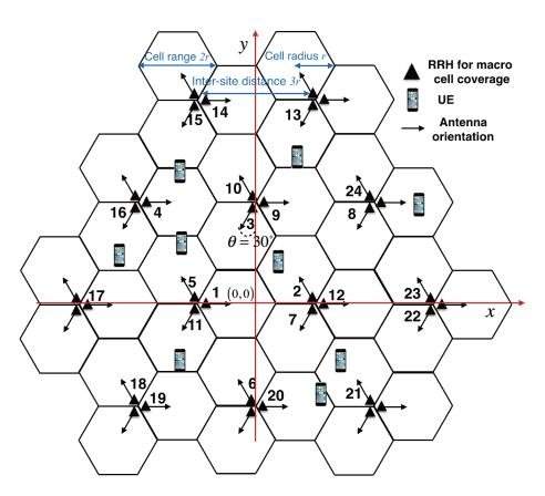
Fig. 4.4 Geometry distribution and clustering of RRHs.
