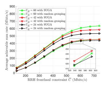
Fig. 7.8 Average achievable sum rate vs. fronthaul capacity constraint  $\overline{C}$  for the UEs served in distributed MIMO mode.
