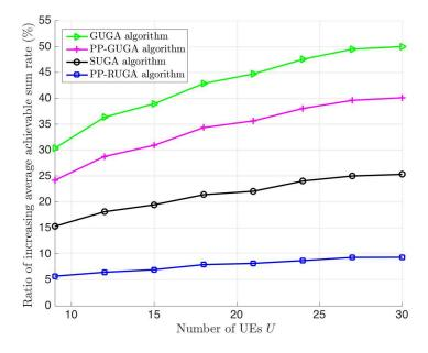
Fig. 6.7 Ratio of increasing average achievable sum rate compared with applying "Random user grouping" vs. number of UEs U ( $P_{\rm dBm}=46$  dBm,  $Q_{\rm q}=4$ ).
