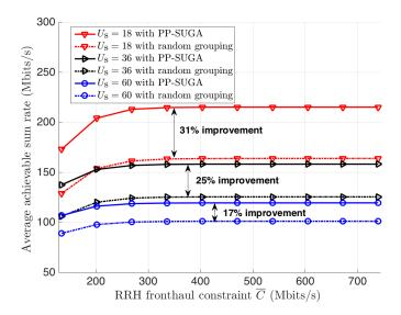
Fig. 7.7 Average achievable sum rate vs. fronthaul capacity constraint  $\overline{C}$  for the UEs served in single RRH mode.
