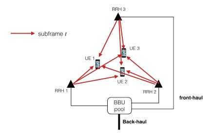
Fig. 5.9 Downlink transmission scheme of distributed MIMO.
