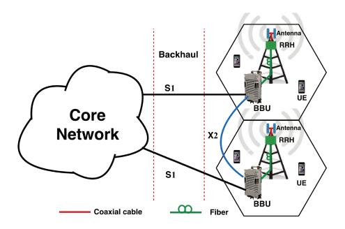
Fig. 2.11 LTE radio access network architecture.
