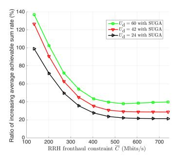
Fig. 7.9 Ratio of increasing average achievable sum rate compared with applying "Random user grouping" vs. fronthaul capacity constraint  $\overline{C}$  for the UEs served in distributed MIMO mode.
