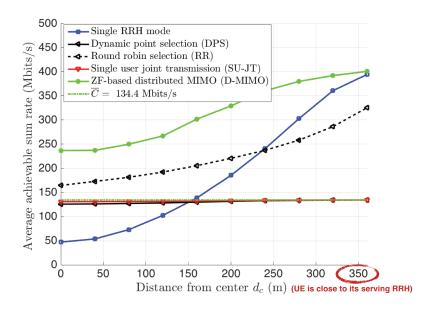
Fig. 5.15 Average achievable sum rate vs. UE distance from the center of RRH 1, 2 and 3  $d_c$  ( $P_{\rm dBm}=41.4$  dBm,  $\overline{C}=134.4$  Mbits/s).
