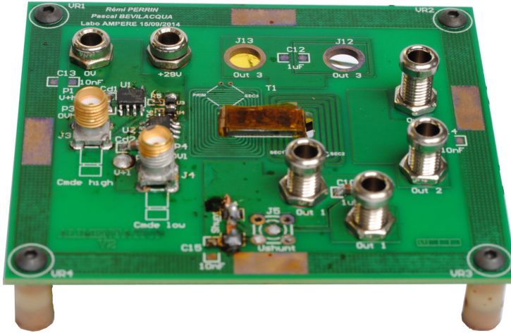
Figure 3.53 – Double output active-clamp flyback prototype with EPC GaN HEMT for high-temperature operation.
