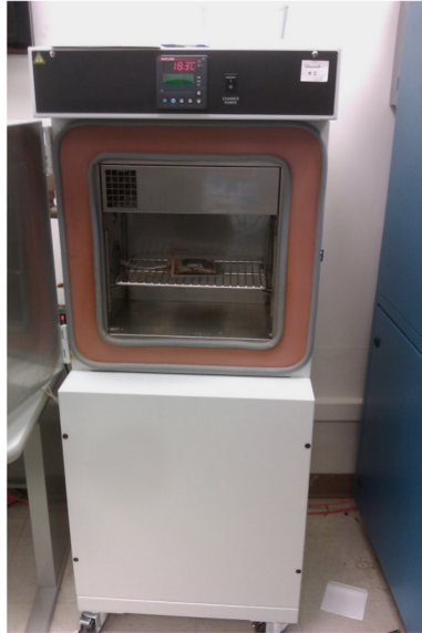
Figure 3.50 – Thermal chamber for the cycling test.
