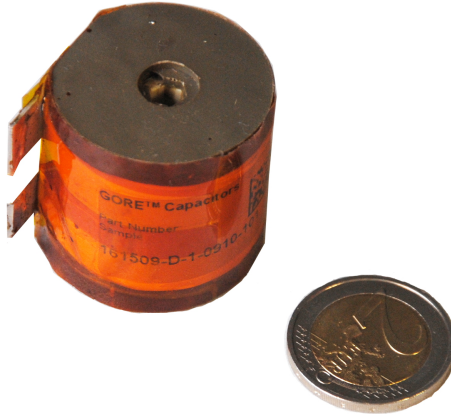
Figure 4.33 – 7 \mu\text{F} 600 V PTFE Gore Capacitor.
