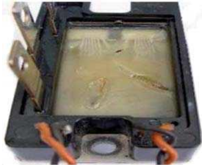
Figure 8: Power module covered with insulating silicone gel [Ménager'10]
