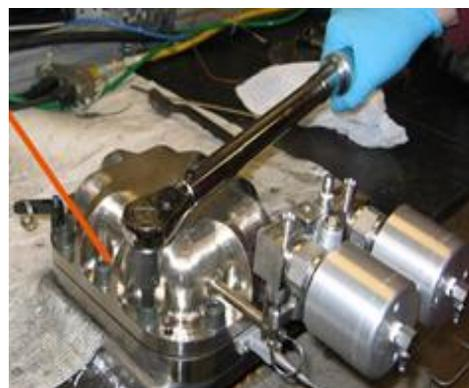
Figure 19: Sealing of the reactor vessel
