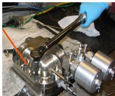
Figure 19: Sealing of the reactor vessel
