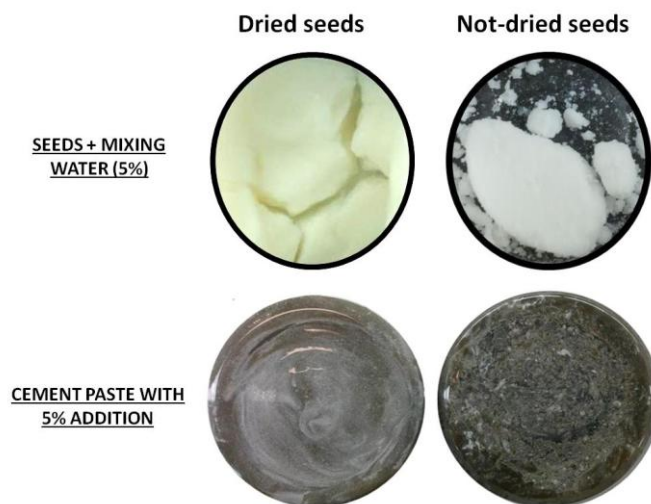
Figure IV.2-1: Comparison between the texture of the seeds mixtures and the cement pastes when the seeds are added dried or not dried.
