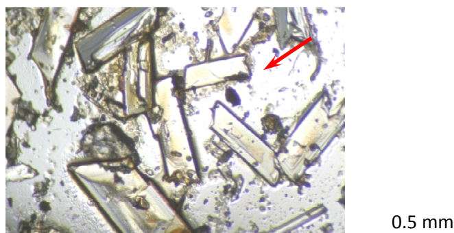
Fig. 56 The picture of crystal forms of product 24 , the single crystal chosen for experiment is marked with an arrow
