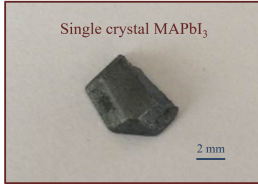
Figure 4.1: A photo of single crystal MAPbI 3 sample. The scale bar is 2 millimeter.
