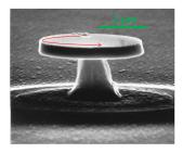
(a) Idea of WGMs: The light beam circulates and then returns to its initial position with the same phase.
