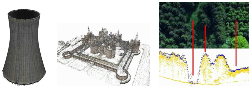
Figure 2.6: 3D model of an air cooler (left, source: SIXENSE Mapping), 3D model of Chambord castle (center, source: ENSG) and canopy model (right, source: [Lisein 2016])
