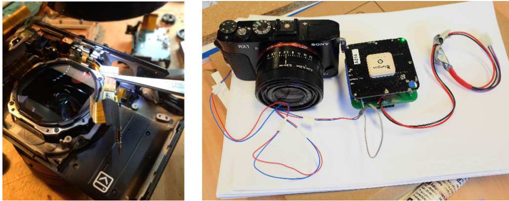
Figure 4.12: Adapting Sony-RX1 camera triggering to GPS module TimePulse feature
