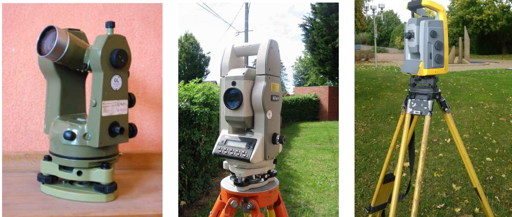
Figure 3.1: Evolution of stations in topometry. Theodolite (right), tachometer (center) and total station (right)
