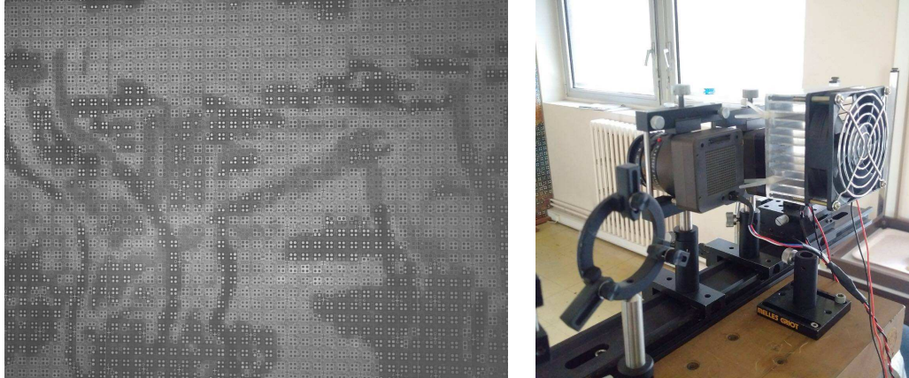
Figure 5.3: The scene of the textured wall (left) and the installation of cameras and peltier cooler (right)
