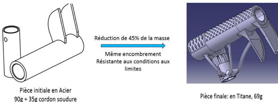
Figure 3-29: Reconcepting a part using our additive manufacturing design process
