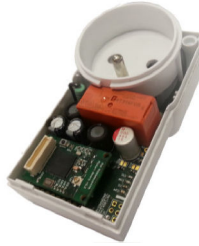
Figure 4.7: The smart plug from Homadeus (a company developing embedded systems).
