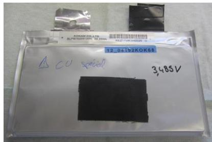
Figure II-1 : 16 Ah commercial Li-ion cell (Kokam SLPB 78205130H).
