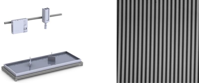
Figure 8.7 – Setup of the profilometry of the gravito-capillary wave experiments of Cobelli *et al.* (2009) and Leoni *et al.* (2015). Left) Scheme of the experimental setup. Right) Sample image of the fringes projected onto the liquid surface as registered by a camera. The figures are extracted from [98, 96].
