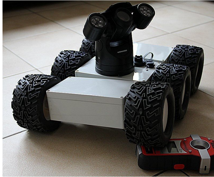
Figure 4.2: Sample photo of Wifibot-M 6-wheels mobile robotic platform
