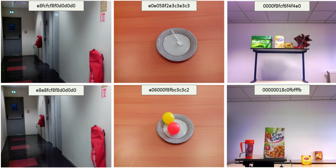
Figure 3.10: Some images from our datasets with corresponding perceptual hashes. Left column shows two almost identical images, center column represents two images with one different region in center, and right column provides two images which show different environment yet in the same room
