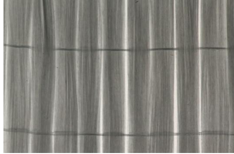
Figure 74 Unidirectional stitched fabric - Tissa
