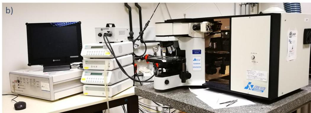
Figure II-35 a) Scheme with Rayleigh and Raman scattering representation<sup>25</sup>; b) Jobin Yvon/Horiba LabRam spectrometer in LMGP
