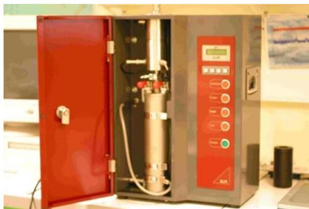
Figure 2.13 : Electrical Low Pressure Impactor (Dekati Inc.).
