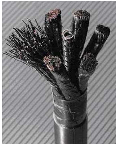
Figure 1-10: Burst representation of a cable in conduit with its six petals
