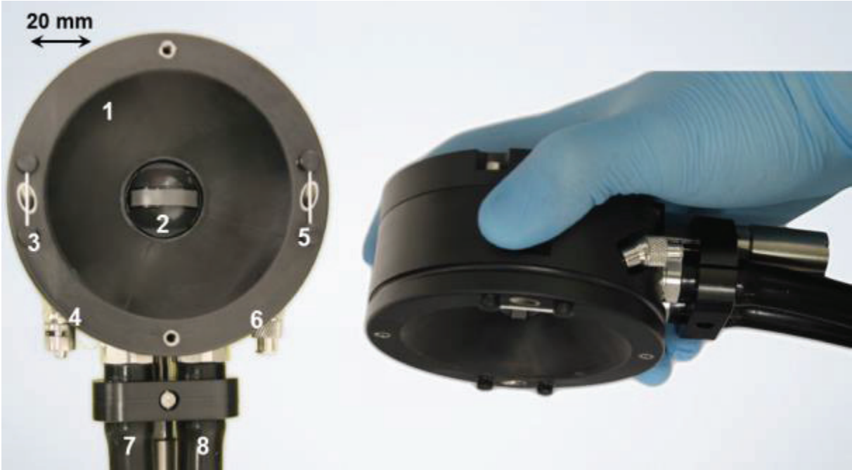
Figure 1. Picture of the HIFU toroidal device. 1: HIFU transducer divided into 32 concentric rings. 2: Ultrasound imaging probe. 3 and 5: Holes for the cooling water. 4 and 6: Connectors for the cooling circuit. 7: coaxial cables for the HIFU emitters. 8: Cables for the ultrasound imaging probe.
