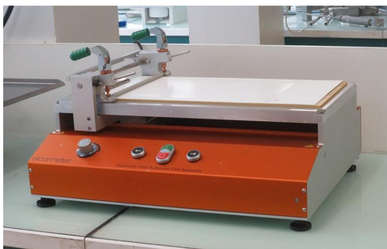
Figure 29 - Elcometer laboratory coater used for composite coating.
