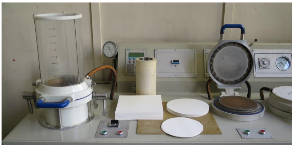
Figure 24 - Rapid-Köthen apparatus for the production of MFC handsheets.
