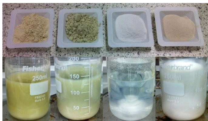
Figure 57 - Pictures of layered silicate powders (top) and suspensions (bottom). From left to right: Cloisite-Na (C), Nanofil 116 (N), Laponite (L), and Kaolinite (K).
