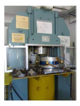
Figure 2.1: The multianvil 1000 tons Walker-type press at IMEM-CNR (Parma, Italy)
