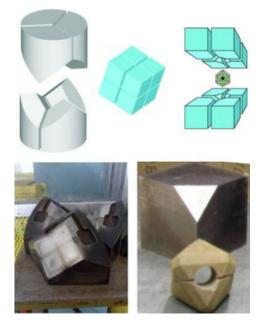
Figure 2.2: up: Scheme of components constituting the Walker type module and the way they are assembled. In the lower part of the figure: from left to right some tempered wedges, a tungsten carbide cube and a correspondent MgO octahedron.
