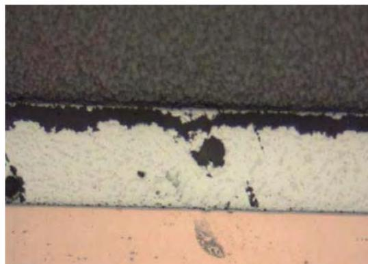
*Figure I.59: Solder fracture due to creep–fatigue under thermal cyclic load [42].*
