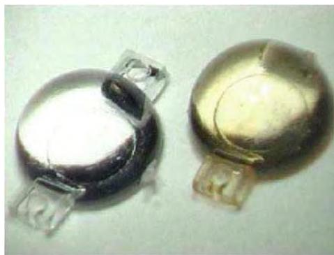
Figure I.54: Encapsulant yellowing [42].
