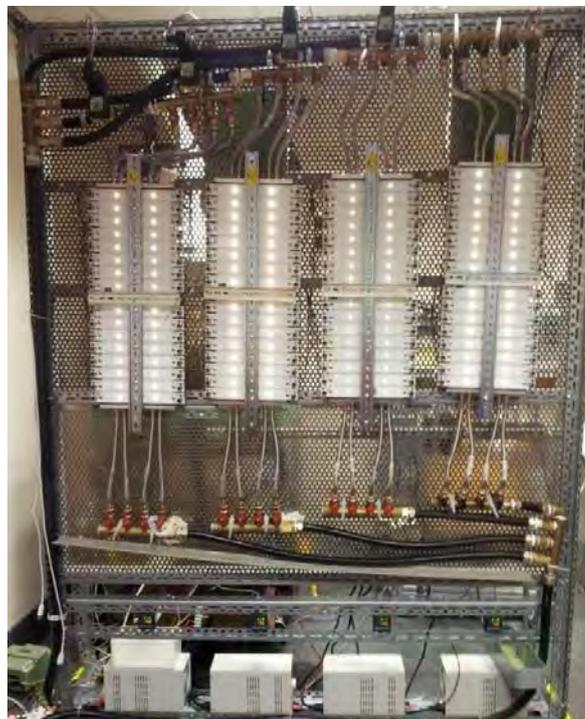
*Figure III.1: Overview of the LED aging Bench.*
