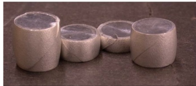
Figure 1.41: Deformed specimens with different ratio of diameter and height ( \eta = -0.33 to -0.05 ) [68]
