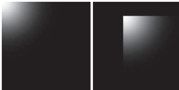
Fig. 7.12.: Cornered Gaussian function without and with shifting. Discontinuities appear on the shifted function that did not exist in the original function.
