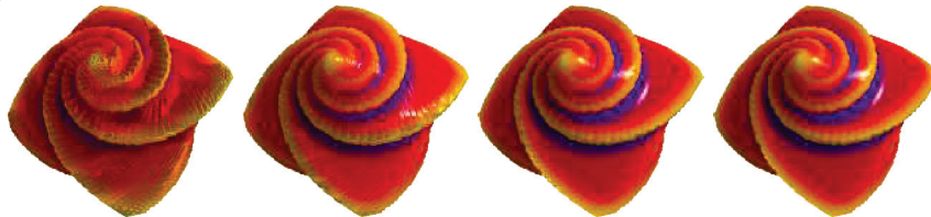
Fig. B.7.: Illustration of mean curvature computation on “OctaFlower” (digital domain of 130^3 ) using mipmap approximation with different levels: l_3 , l_2 , l_1 and l_0 ( i.e. no approximation).
