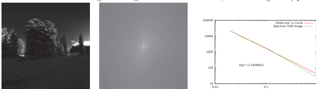
Results from a HDR Image showing a natural scene, with an O(\rho^{-1.59}) profile.
