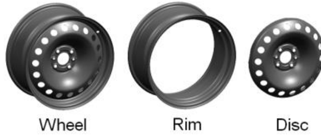
Figure 2.1: Image of the wheel and its two main components
