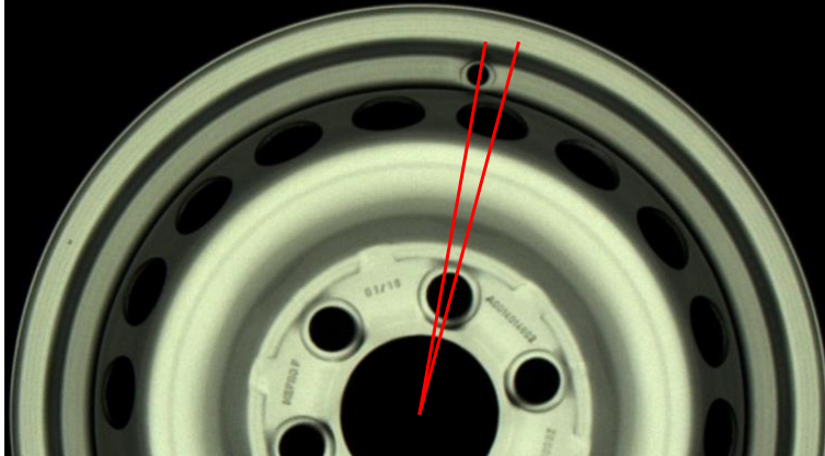
Figure 2.5: An example of a dimensional defect on the surface of the wheel
