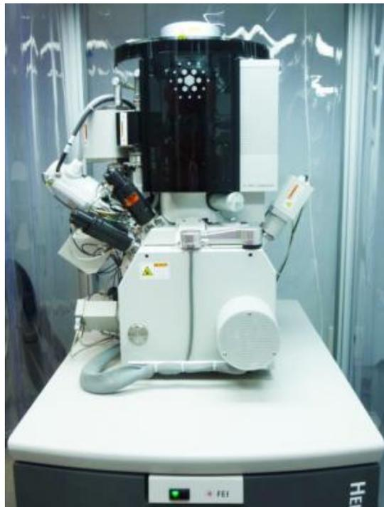
Figure 2.4: Dual Beam SEM/FIB equipment (FEI Helios 600i).
