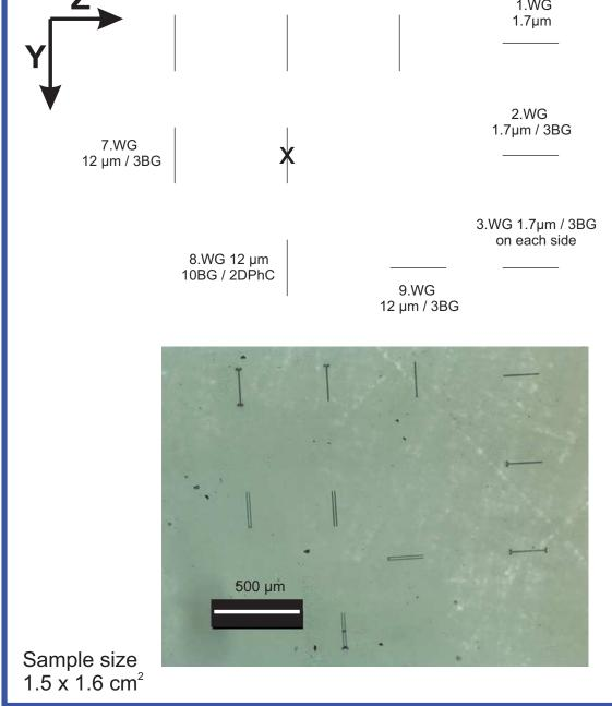
Figure 7.10: Sketch of the waveguides positions on the sample surface and the microscope image of fabricated structures.
