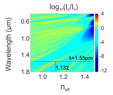
Figure 7.2: Dispersion curve for designed 1DPhC.
