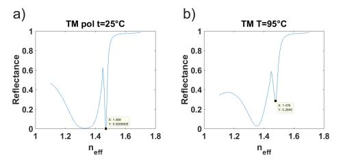
Figure 7.18: (a) Reflectance for the multilayer with VO<sub>2</sub> at 25°C temperature; (b) Reflectance for the multilayer with VO<sub>2</sub> at 95°C temperature.
