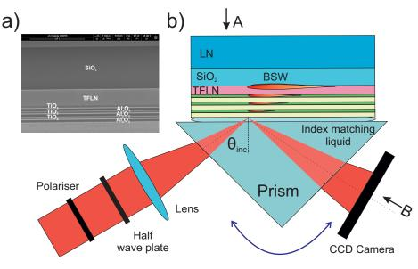
Figure 5.6: (a) FIB-SEM image of 1DPhC; (b) Experimental set up.
