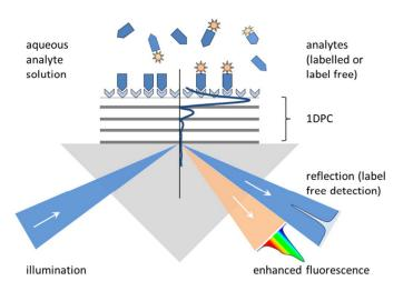
Figure 1.2: Scheme of a Bloch surface wave optical biosensor for label-free and fluorescence detection [43].
