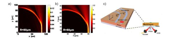
Figure 1.6: Experimental (a) and theoretical (b) intensity distribution of bending waveguides having different radii values.  $R=80\mu m$ . (c) Schematics of BSW coupling into the curved waveguides[4].
