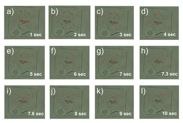
Figure 4.6: (a) Sample visualization with x20 objective; Illustration of the grating, latex beads and rectangular shape of the incident beam; Demonstration of beads attraction by focused light (a-g); Illustration of beads, pushed away from the grating by BSW (g-i).
