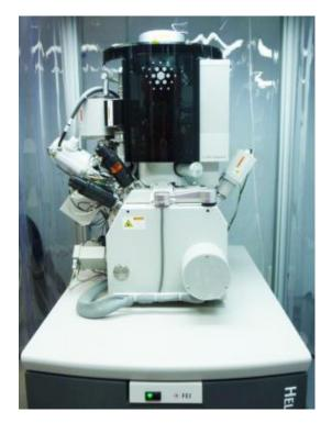
Figure 2.4: Dual Beam SEM/FIB equipment (FEI Helios 600i).
