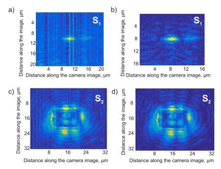
Figure 3.20: (a)Data from original image around the grove area; (b) Data from original image around the grating area; (c) Processed image without the noise for the grove area; (d) Processed image without the noise for the grating area.
