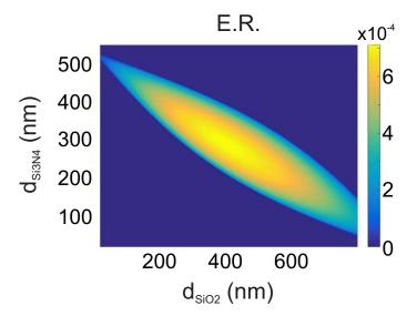
Figure 7.1: Extinction of the band gap as a function of layer thicknesses in 1DPhC.
