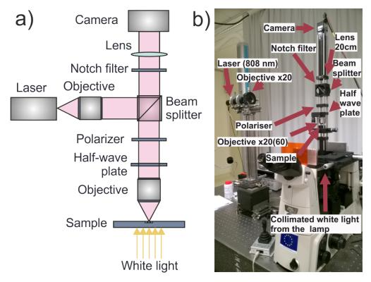
Figure 4.5: (a) Schema of experimental setup for sample characterization; (b) Optical table with the setup.
