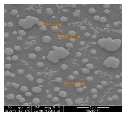
Figure 6.13: SEM image of the TFLN surface of the sample on glass support after Si and  $SiO_2$  removal with DRIE, RIE and additional 57 min in BHF.
