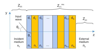
Figure 2.1: Reflection and transmission for a multilayer with N layers.
