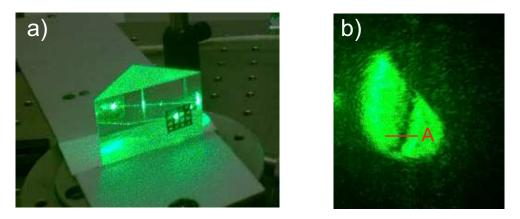
Figure 6.9: (a) BSW excited on the sample with matrix of 16 membranes in Kretschmann configuration; (b) Image of reflected light at the BSW coupling angle collected by camera for the membrane. A - selected line for the image cross-section.
