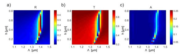
Figure 3.8: (a) Reflection  $R(\Lambda, h)$ ; (b) Transmission  $T(\Lambda, h)$ ; (c) Absorption  $A(\Lambda, h)$  as a function of period and width of the grooves. Depth is equal to width.
