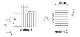
Figure 3.3: Polarization with respect to gratings
