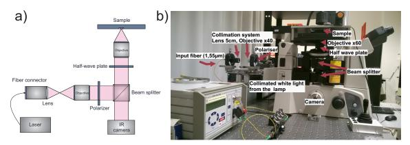
Figure 3.12: (a) Schema of experimental setup for sample characterization; (b) Optical table with the setup.
