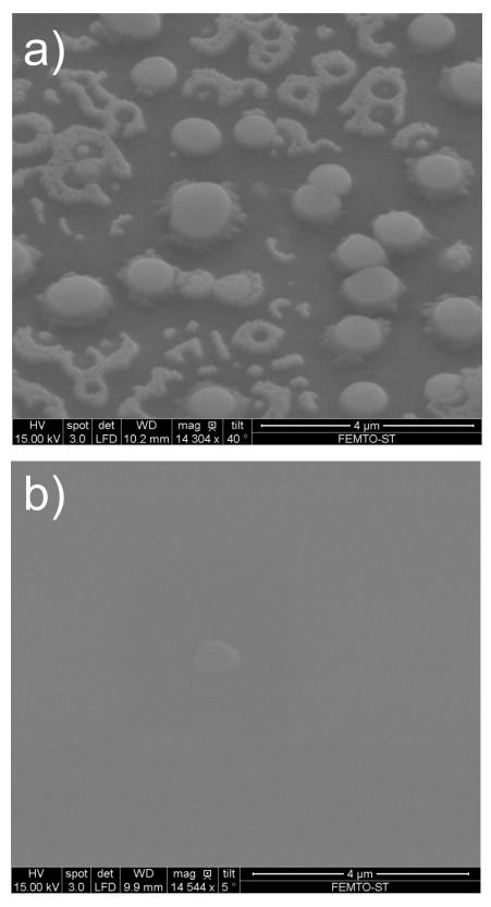
Figure 6.15: SEM images of 1DPhC with TFLN top surface before (a) and after (b) implementation of additional cleaning and temperature stabilization protocols.
