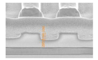
Figure 3.6: FIB-SEM image of the analytically optimized grating cross-section for the Sample 1
