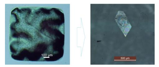
Figure 6.16: (a) Single TFLN membrane suspended in air; (b) TFLN membrane transported to the microscope cover glass.
