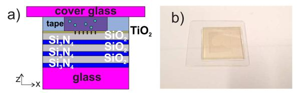
Figure 4.4: (a) Schematics of the sample with a chamber; (b) Sample with a chamber and solution with beads in the chamber.
