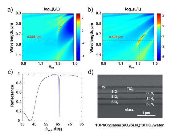
Figure 4.2: (a) Band gap diagram of the 1DPhC without  $TiO_2$ ; (b) Band gap diagram of the 1DPhC with  $TiO_2$ ; (c) Calculated reflectance at 808 nm wavelength; (d) FIB-SEM image of 1DPhC.
