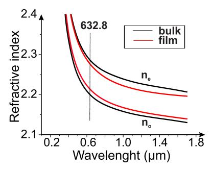
Figure 5.2: Measured refractive indices for LN bulk and TFLN.
