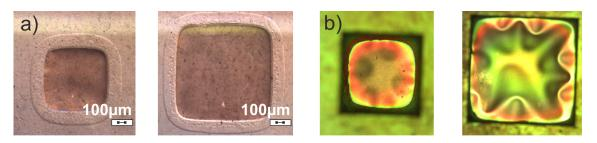
Figure 6.3: (a) The microscope images of the membranes. (b) The microscope images of the membranes after multilayer deposition.
