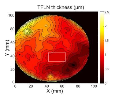
Figure 6.1: The thickness profile of the TFLN.
