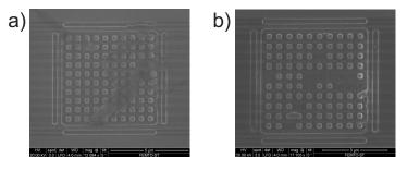
Figure 4.8: (a) Grating contamination by glue from the tape after the forth cleaning time; (b) Burned or broken grating after the sixth cleaning time. After several times reusing the sample, grating still can get contaminated up to the point that it is impossible to clean [Fig. 4.8(a)] or can even get broken [Fig. 4.8(b)].
