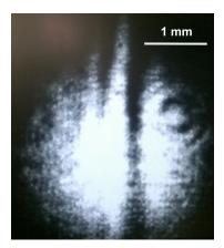
Figure 7.6: Image of reflected light at the BSW coupling angle collected by IR camera (the image is almost the same for the samples with 4, 5 and 6 pairs of  $Si_3N_4$  and  $SiO_2$ ).
