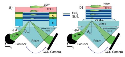
Figure 6.7: (a) Experimental setup for the on-membrane 1DPhC. (b) Experimental setup for the on-glass 1DPhC.
