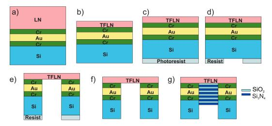
Figure 6.2: Schematic of the membrane based 1DPhC fabrication process: (a) Bonding of bulk  $LiNbO_3$  to Si with Cr and Au, (b)  $LiNbO_3$  polishing, (c) Photoresist deposition, (d) UV lithography of the photoresist, (e) DRIE etching of Si and wet etching of Cr and Au, (f) Photoresist removal, (g) Multilayer deposition.
