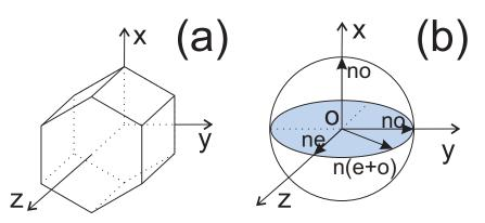
Figure 5.1: (a) Sketch of the crystalline directions of LN; (b) Sketch of index ellipsoid of LN.
