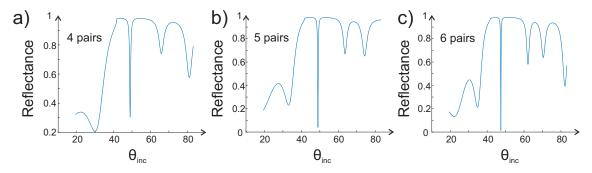
Figure 7.3: Calculated reflectance in 1DPhC for (a) 4 pairs, (b) 5 pairs and (c) 6 pairs of  $Si_3N_4$  and  $SiO_2$ .
