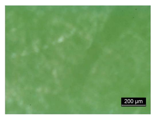
Figure 6.14: Microscope image of the TFLN surface of the sample on glass support after Si and SiO<sub>2</sub> removal with DRIE and RIE.
