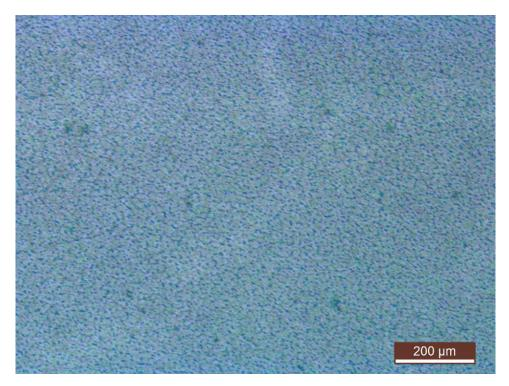
Figure 6.11: Microscope image of the TFLN surface of the sample on glass support after Si and SiO<sub>2</sub> removal with DRIE and RIE.
