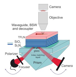
Figure 7.11: Experimental setup for the wave-guiding characterization.
