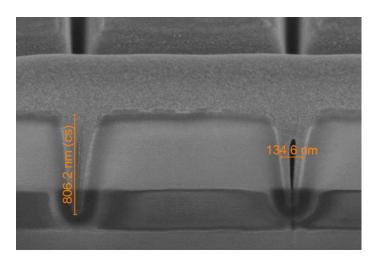
Figure 3.10: FIB-SEM image of the analytically optimized grating cross-section for the Sample 3.
