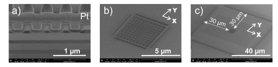
Figure 4.3: (a) FIB-SEM image of the analytically defined grating cross-section for the BSW in water; (b) SEM image of the manufactured grating; (c) SEM image of the final sample for BSW in water.
