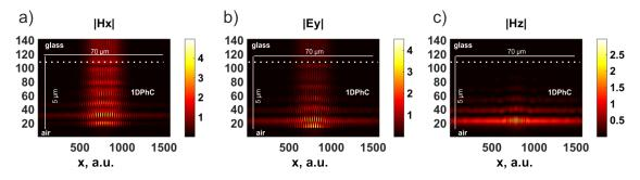
Figure 3.22: Field profile inside the 1DPhC with decoupling ridges for (a)  $H_x$ ; (b)  $E_y$ ; (c)  $H_z$  field components.
