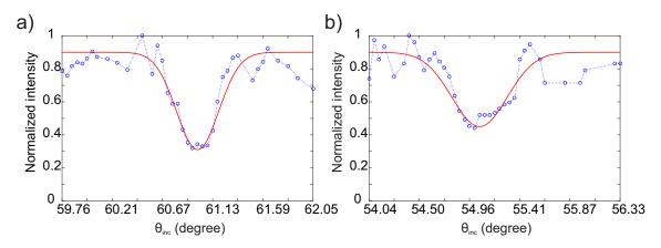
Figure 6.8: (a) Camera image intensity profile of the BSW related reflectance dip for the membrane based sample. (b) Camera image intensity profile of the BSW related reflectance dip for the on-glass sample. In blue - cross-sections of the reflected light images. In red - Gausian fit for experimental data.
