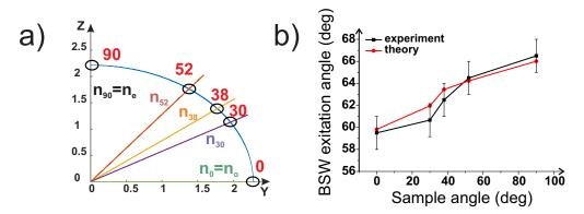
Figure 5.9: (a) Refractive index of LiNbO<sub>3</sub> for different sample positions; (b) Experimental results and theoretical dependance of the BSW excitation angle
