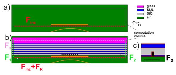
Figure 3.21: (a) System and flux line for input energy calculations; (b) System and flux line for energy coupled to BSW and transmitted (multilayer without groves); (c) System and flux line for decoupled energy.
