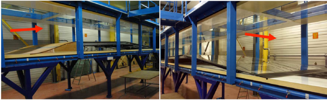
Figure 4.2: The ramp model placed in the LML boundary layer wind tunnel
