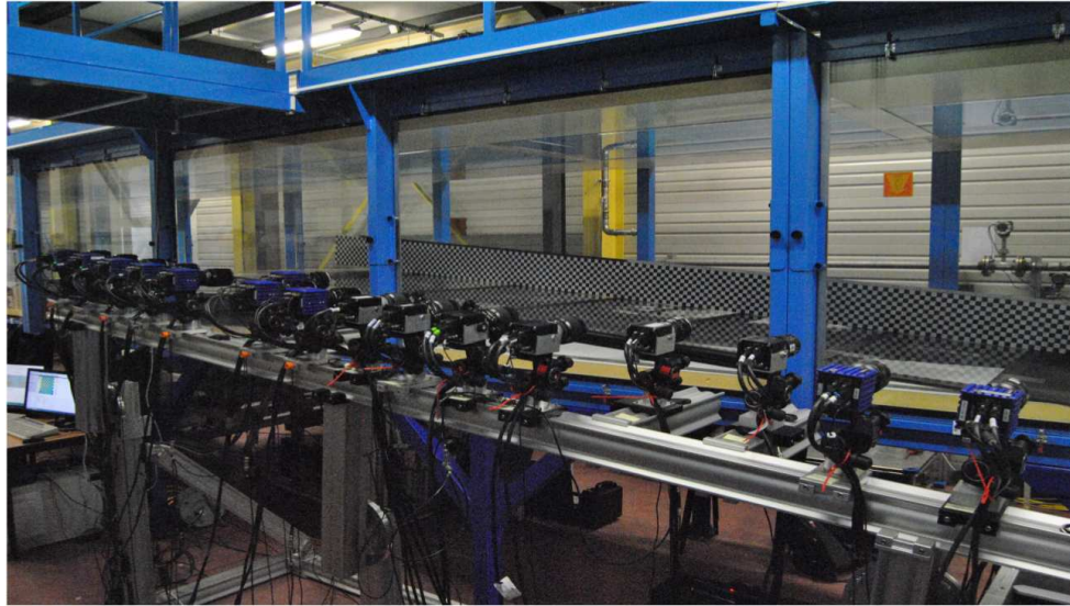
Figure 4.14: The set of 16 sCMOS cameras aligned in series and mounted on the side of the wind tunnel. The target used for calibration is placed along the centerline of the ramp
