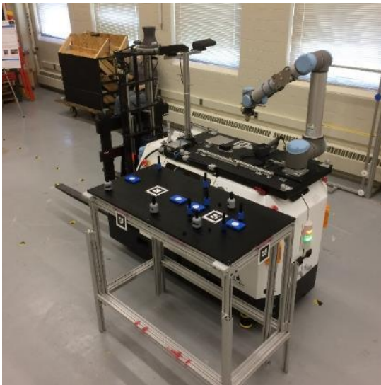
Figure 76. Ten different AGV poses for testing mobile manipulator performance.
