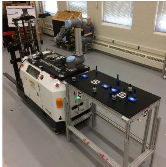
Figure 76. Ten different AGV poses for testing mobile manipulator performance.
