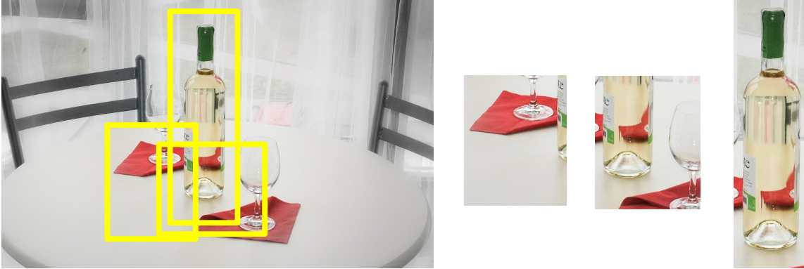
Figure A-2: Reducing the detection task to a classification problem. The goal is to find a tight bounding box around the bottle. We sample possible locations, reducing the task to binary classification predicting whether the input window contains completely and predominantly the object of interest.
