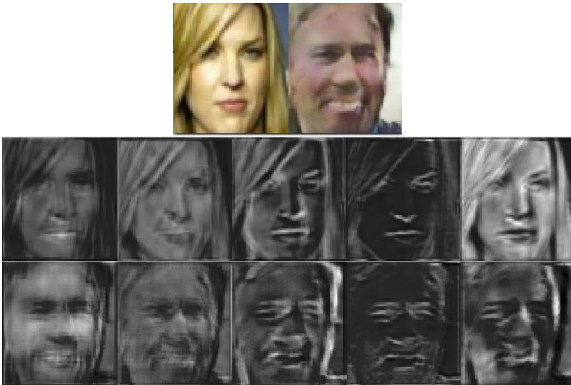
Figure 5-6: First row: Face from the training dataset (left) and face generated by a Deep Convolutional GAN (right). Second row: output maps of the first convolution layer for the real face. Third row: same output maps for the generated face. While the generated face does not show visible artifacts, some appear clearly as horizontal and vertical lines, especially on the two leftmost maps.
