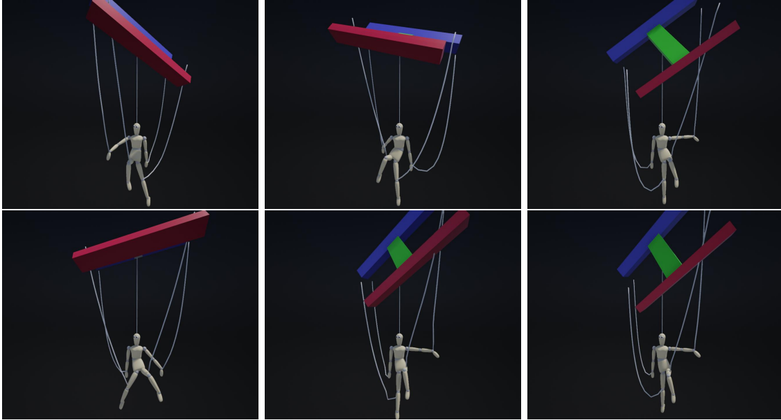
Figure 5-11: Examples from the dataset we built from screenshots of our puppet simulator. The limb configuration of the puppet, attached to the plate with strings, depends on the position of the colored plate.
