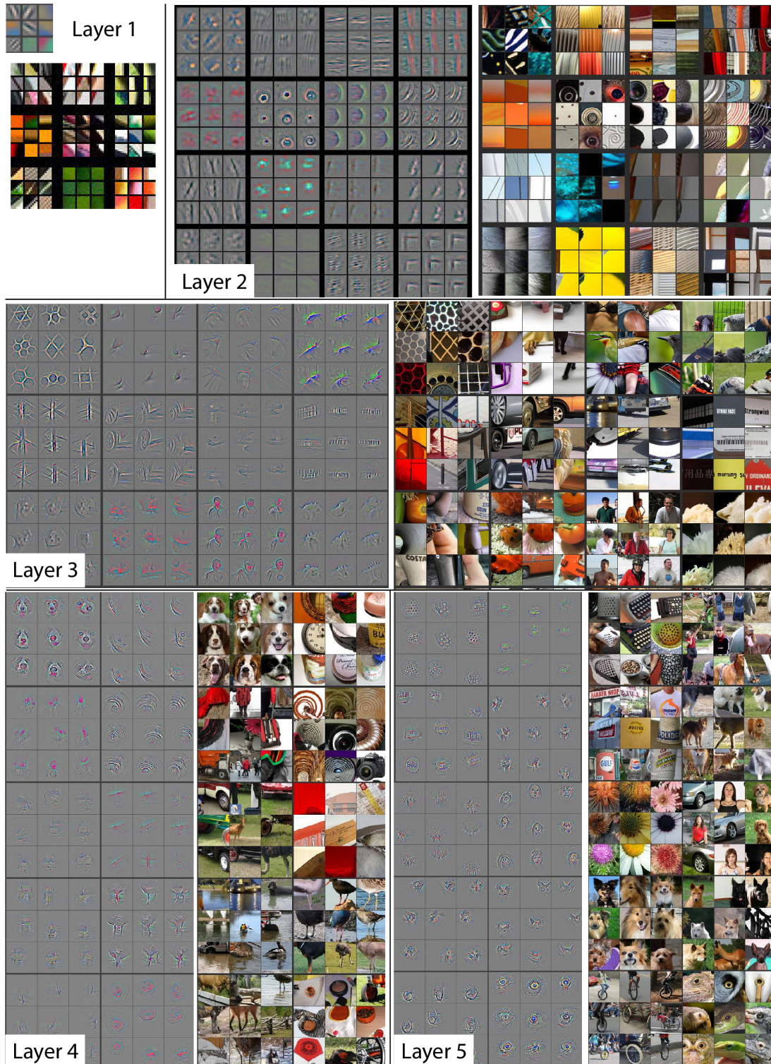
Figure B-24: Original caption: Visualization of features in a fully trained model. For layers 2-5 we show the top 9 activations in a random subset of feature maps across the validation data, projected down to pixel space using our deconvolutional network approach. Our reconstructions are not samples from the model: they are reconstructed patterns from the validation set that cause high activations in a given feature map. For each feature map we also show the corresponding image patches. Note: (i) the strong grouping within each feature map, (ii) greater invariance at higher layers and (iii) exaggeration of discriminative parts of the image, e.g. eyes and noses of dogs (layer 4, row 1, cols 1). Best viewed in electronic form. Figure and caption from Zeiler and Fergus [2014].
