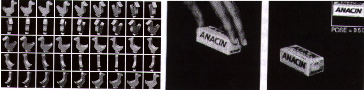
Figure 2-3: Empirical models of image variability, by Murase and Nayar [1995] . They introduce pose invariance in recognition by capturing multiple rotated views of objects. At run-time they recognize objects and the closest rotation angle for that view.
