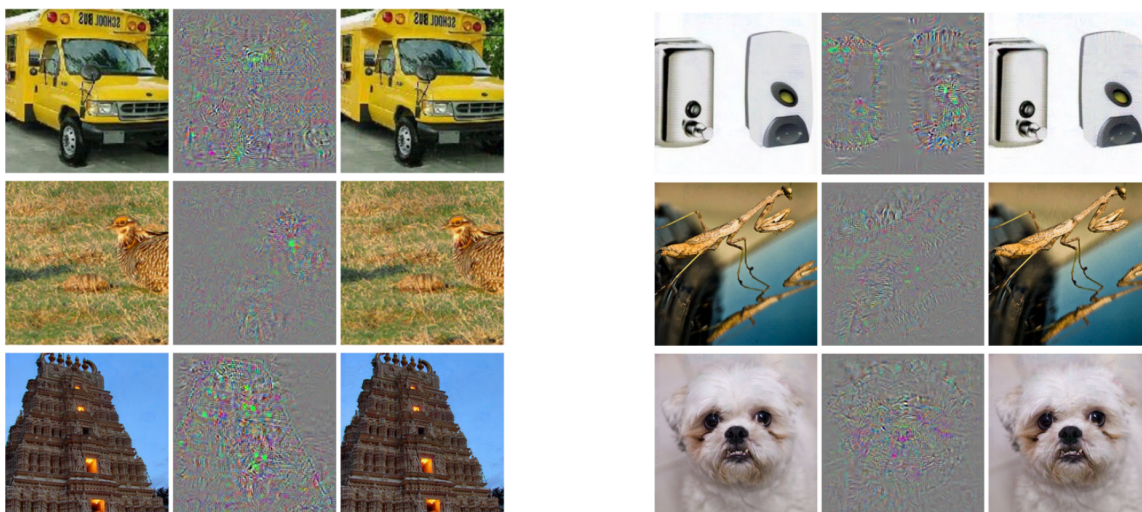
Figure 2-59: Adversarial examples proposed by Szegedy et al. [2013]. Original caption: Adversarial examples generated for AlexNet. (Left) is a correctly predicted sample, (center) difference between correct image, and image predicted incorrectly magnified by 10x (values shifted by 128 and clamped), (right) adversarial example. All images in the right column are predicted to be an “ostrich, Struthio camelus ”. Average distortion based on 64 examples is 0.006508. Please refer to http://goo.gl/huaGPb for full resolution images. The examples are strictly randomly chosen. There is not any postselection involved.
