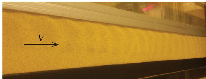
Fig. 10.10 Aeolian sand ripples emerging from a flat bed in the wind tunnel, with the arrow showing the wind direction. Wind velocity at the central of the tunnel is  $V \approx 4.0$  m/s
