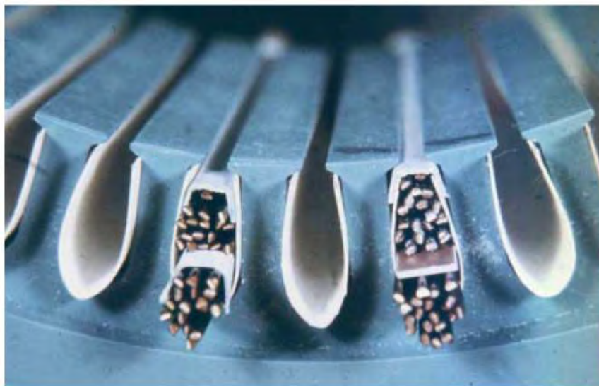
Figure I.5: Slot liner, slot separator, and wedges seen during assembly [13]
