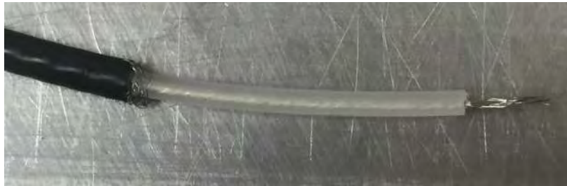
Figure I.20: Sensor based on coaxial cable
