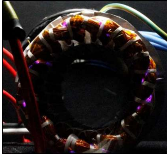
Figure I.7: Partial discharges between phases (100 mbar)
