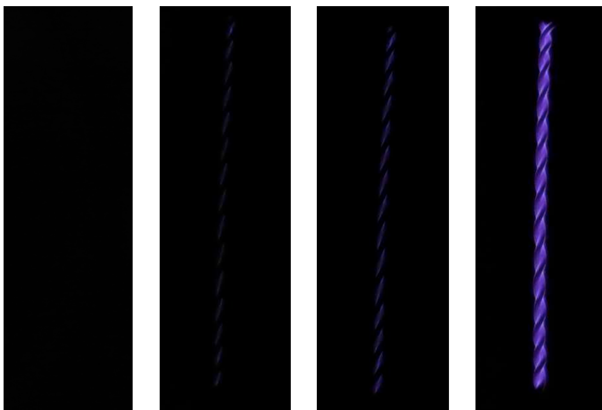
Figure II.29: Influence of the pressure on the “light” emitted by PDs on twisted pair at PDIV for a frequency of 10 kHz
