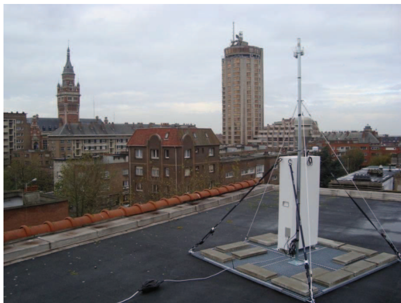
Figure 6 Photo of the A8 big volume sampler location in Dunkerque showing the stabilizing metallic grid on the floor holding about 15 kg of cement.
