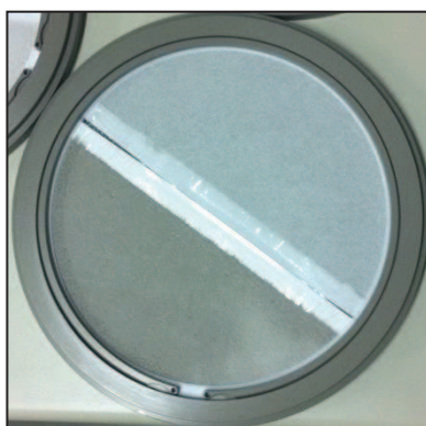
Figure 8 Sample of a sample taken using the A8. The darker side represents the quartz semi-filter and the other lighter one is the cellulose semi-filter. Adhesive tape can be seen in the middle.
